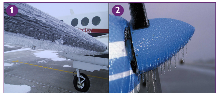
Accumulation of frozen rain droplets (ice) and snow on (1) aircraft wings and (2) propeller and engine parts.
