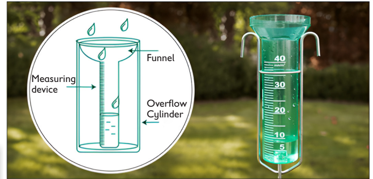
Parts of a rain gauge.
